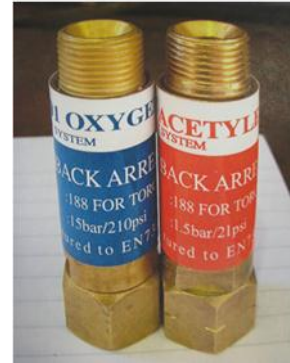
Non-compliant flashback arrestors identifiable only by attached stickers.
